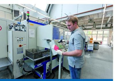
Following the diverse processing steps such as machining, grinding and coating, the parts undergo cleaning in solvent-based systems. The specific cleaning program is selected via bar codes.
