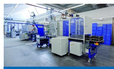
Multiple solvent-based systems are used at the pre-cleaning level in order to separate material flows and to prevent cross-contamination.
