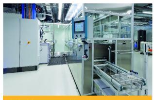
The final cleaning system delivers the product directly into the cleanroom. The system and its conveyor unit are fully enclosed all the way into the cleanroom.
