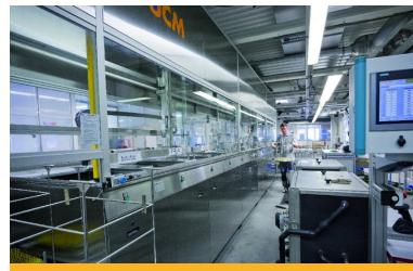
The first stage of the ultrasonic cleaning system used for final cleaning has three separate tanks. Parts consisting of different materials can thus be cleaned separately.
