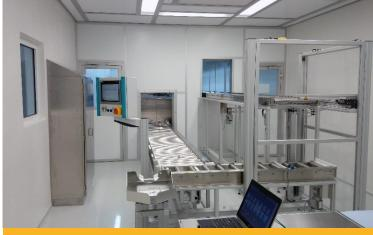
The cleaned parts exit into a cleanroom through an airlock
