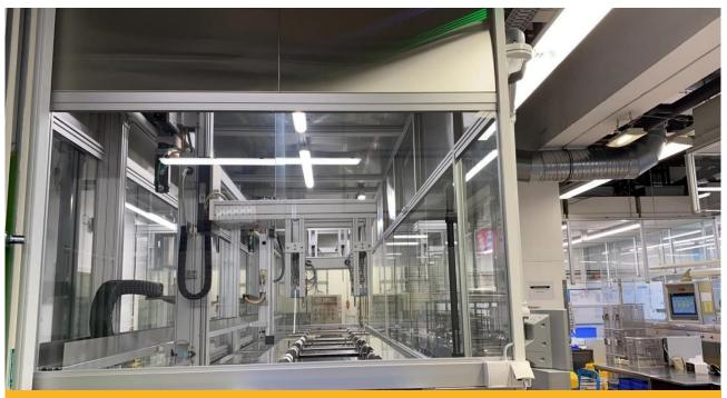
The transport racks of the two transfer units have different grippers to pick up the various cleaning containers provided by the customer and carry out program-specific movements of the containers in the treatment stations.
