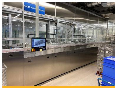
The ultrasonic fine cleaning system, equipped with twelve treatment stations, ensures that the cleanliness specifications of two or less particles of 5 μm or one or less particle of 10 μm are reliably met when X-ray tube parts receive their final clean.
