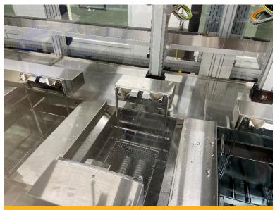
The integrated spray rinse with deionized water removes even very fine dust particles still sticking to the surface after cleaning and the first immersion rinse.
