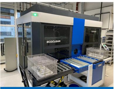
The components of spiral groove bearings are to be cleaned in a standard machine. Cleaning tests before the investment showed that only the EcoCwave can achieve the required results.
